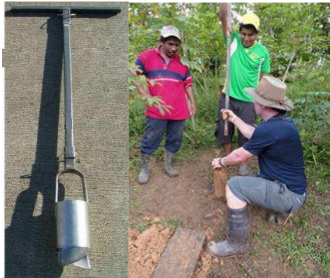
Figure 4: (a) Hand Auger (b) Hand Auger in Operation, Detaching Bit to Remove Soil
