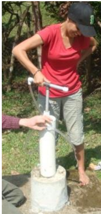
Figure 8: EMAS Hand Pump in Operation
